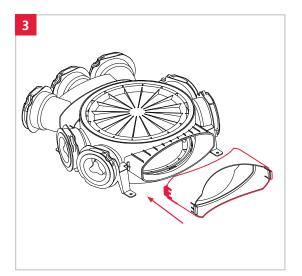
2 Make sure that the seal at the socket is properly placed, if not, correct it. If you notice that the seal is damaged, contact the distributor for a replacement. Dampen the seal with water to reduce friction.
