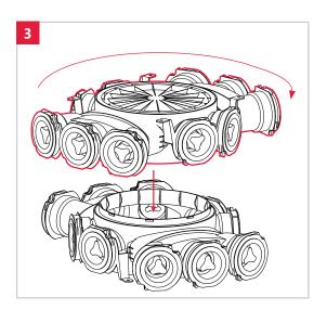
2 Insert the vertical coupling into the uncovered socket of the bottom distribution box. Check if the coupling properly entered the socket and turn it clockwise until the end.
