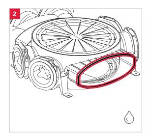
4 Slide the second distribution box into the horizontal connector **Done!** If needed, you can join more distribution boxes together.
