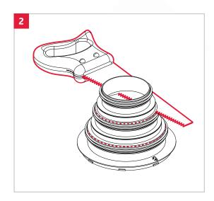
Installation of main connector for inlet/ exhaust air. Type 2: side connector 75mm/90mm.
