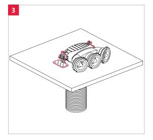
5 Take out the end cap from the socket, put the seal on the first furrow of the pipe and slide the pipe into the socket. Make sure that the fastening ring is in the locked position. When installing two pipes, use two outer sockets, one pipe - the middle socket. Unused sockets have to remain capped.
