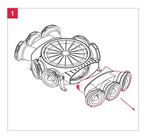
Slide the horizontal coupling on the eliptical slot of the first distribution box. Check if catches are properly fastened.
